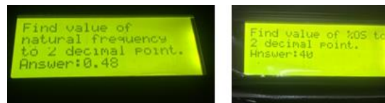
Figure 5 4 20x4 LCD shows the questions asked to find natural frequency and %OS value.
